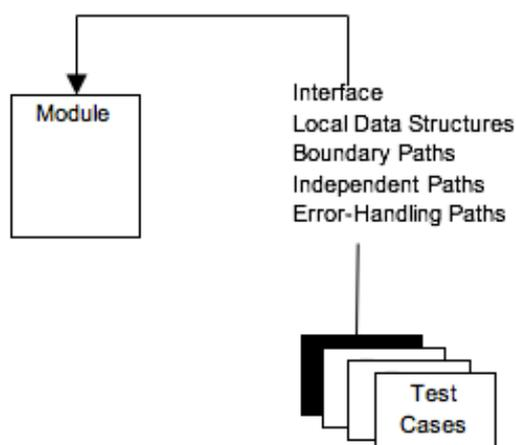
Figure 4.4: Unit Tests (Source: Agarwal et al., 2010)
